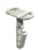
The push-fit anchor can accept a cable tie (type 550 or 555) up to 9 mm wide, which can be used to install several cables and pipes. Suitable for concrete, lime sand and brickwork as solid brick. Use in gas concrete masonry is possible, but reduced load capacities must be expected.
