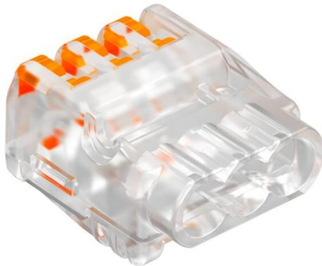
Electrical connections are made with screw-in and screwless terminals. In terminal strips and Dolü branch terminals, the cables are fixed in the terminal using a screw. With screwless terminals, the contact and the holding force is applied to the wires using special spring mechanics. The transparent cover of the contact terminals allows a visual check of the correct wire connection in the screwless terminals.
